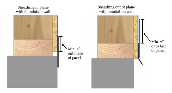
Note: LP WeatherLogic Seam & Flashing Tape must extend at least 2" onto the face of the LP WeatherLogic panel. LP does not require the tape to adhere to the masonry foundation.
