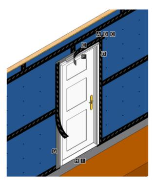
Door unit has flashing tape applied between brickmold and door jamb to create flashing flanges
