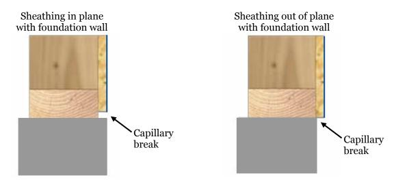
Note: Install a capillary break between the foundation and sill plate as required by code.
