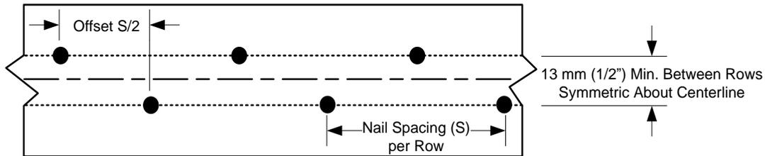
Figure 1. Spacing of multiple rows of nails.
