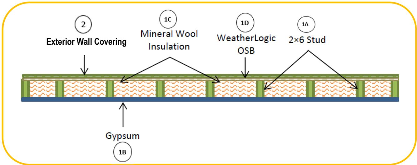
1. **WALL ASSEMBLY:** Construct a 1 hour rated gypsum wall assembly, with resistance from either side using the following elements:
