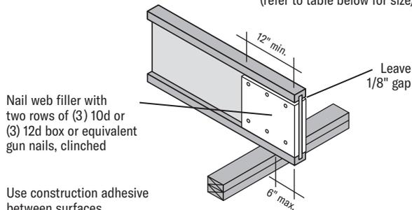
Nail web filler with two rows of (3) 10d or (3) 12d box or equivalent gun nails, clinched
