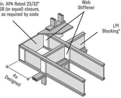
\* LP SolidStart Rim Board, LVL or LSL may be substituted for the LPI Blocking
