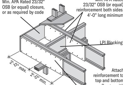
\* LP SolidStart Rim Board, LVL or LSL may be substituted for the LPI Blocking
