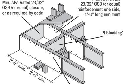
\* LP SolidStart Rim Board, LVL or LSL may be substituted for the LPI Blocking
