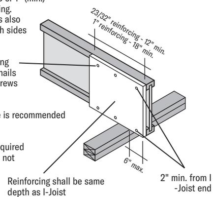
Reinforcing shall be same depth as I-Joist
