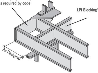
\* LP® SolidStart® Rim Board, LVL or LSL may be substituted for the LPI Blocking
