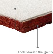
Look beneath the ignitionresistant Pyrotite<sup>®</sup> coating and you'll find the strength of LP<sup>®</sup> OSB.
