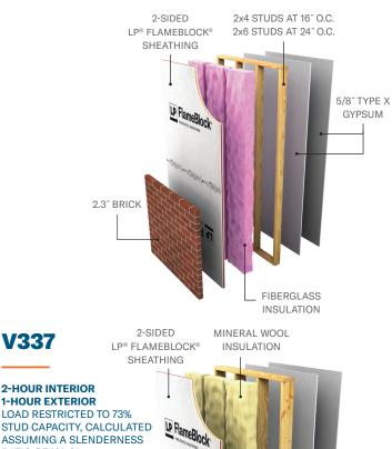
**1-HOUR EXTERIOR** LOAD RESTRICTED TO 73% STUD CAPACITY, CALCULATED ASSUMING A SLENDERNESS RATIO OF I/d=21
