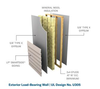
1-Hour Fire-Resistance-Rated Wall; Fire-Rated Either Side
