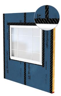
Improper sequencing results in the upper seam tape running under the head flashing. This provides a direct path for water along the edges of the seam tape under the head flashing, which can then leak into the wall.
