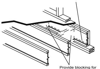
lateral support as required. Use LP I-Joist, LP LVL, LP LSL, or LP Rim Board as blocking
