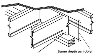
10d box nails at 6" oc toe-nailed from side away from I-Joists
