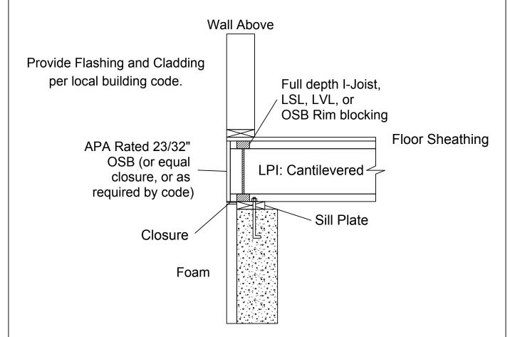
Verify Cantilever Capacity. No Cantilever Reinforcing is required when the full depth blocking (LPI, LSL, LVL, or OSB) is completely: under the wall above, and above the sill plate below. Designer is responsible for verifying that the blocking is capable of transfering all loads (both vertical and lateral).
