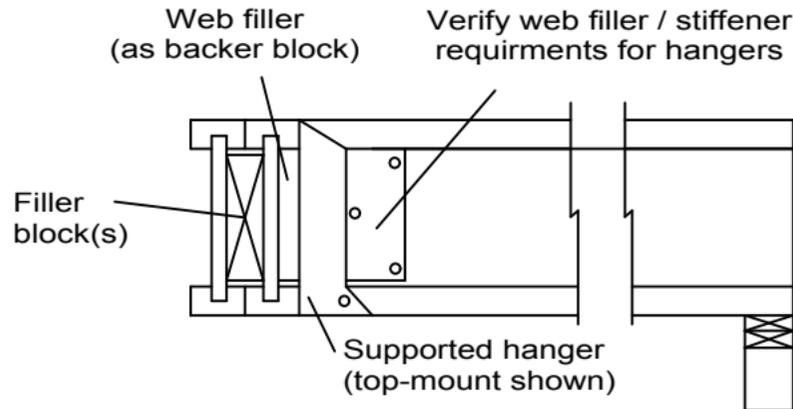
**Web Filler/Backer Block:** Backer blocks shall be at least 12" long and located behind every supported hanger. For a single I-joist header, install backer blocks to both sides of the web. Two pieces of 2 x 8 (min.) lumber, cut to the proper height (see notes 2 & 3), may be set vertically side-by-side to achieve the required minimum 12" length.
