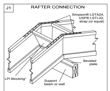
\* Lateral resistance shall be provided. Other methods of restraint, such as full depth LP SolidStart OSB Rim Board, LP SolidStart LVL, LP SolidStart LSL or metal X-bracing may be substituted for the LPI blocking shown.
