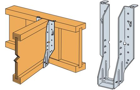
Face mounted joist hanger for supporting I-joists from timber members. Backer blocks required.
