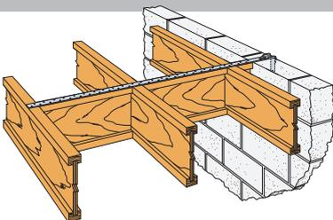
Replaces traditional 5mm heavy restraint strap. Being only 1.5mm thick allows the strap to span over the top of the joists without the need for notching.
