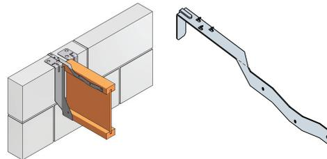
Horizontal restraint strap that provides restraint at every joist. For use with joist spacings up to and including 600mm c/c.
