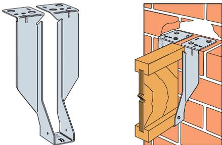
Joist hanger for supporting I-joists and beams from masonry walls.
