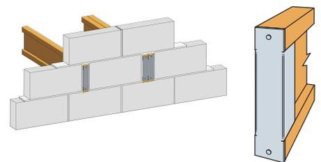
Designed to be used where I-joists are built into masonry walls, to help solve air leakage problems associated with shrinkage of timber and masonry.
