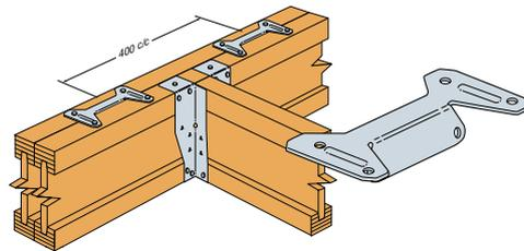
MJC's allow two joists to be fixed together to act as a single unit, replacing the traditional filler block. MJC fitted top and bottom of joists.
