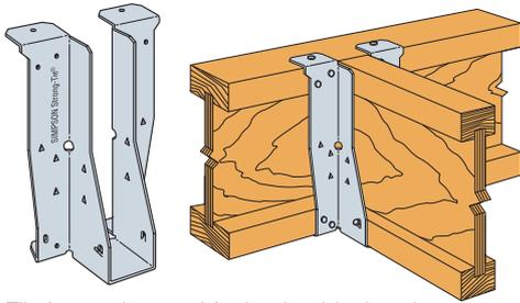
Eliminates the need for backer blocks when supported from an I-joist header.
