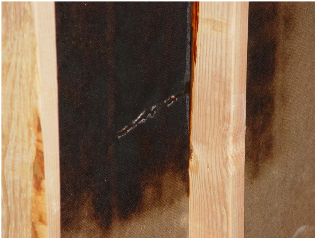
Series 2, Test 8, Slight glowing nonfire side near test termination, IR camera shows diminishing temperature
