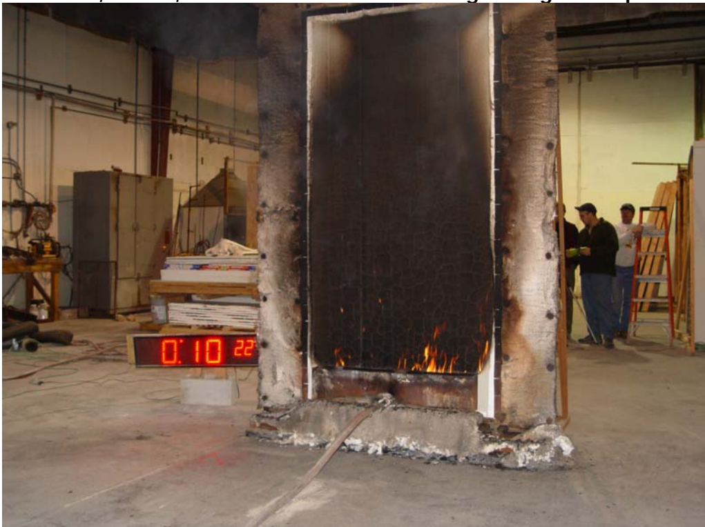
Series 2, Test 8, SmartSide Hardboard siding, fire side, immed. After fire exposure
