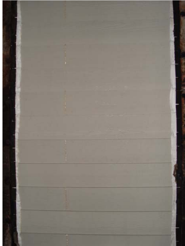
Series 4, 1/2" LP Smartside® Foundation Series exterior lap siding – wet process fiber back-bone, 8" wide, 1" overlap, 16" face nailing, applied over 1/2" standard fiber glass faced exterior grade gypsum sheathing (reference WFCi P/N 07058, Tests 7, 8 & 9)
