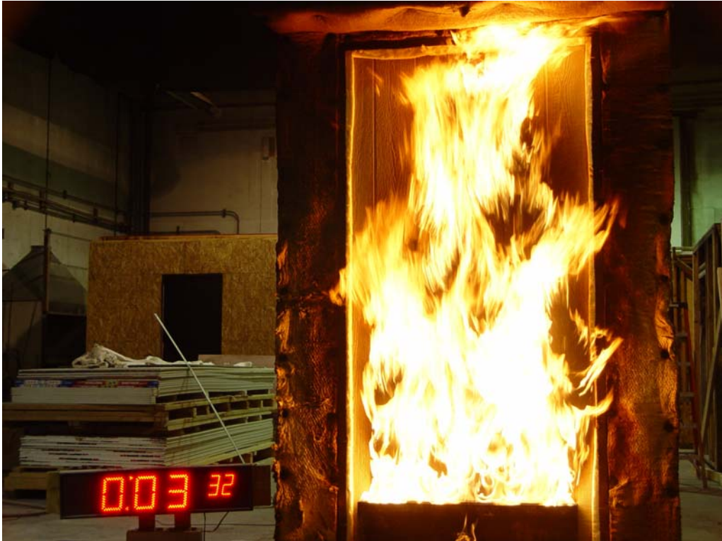
Series 2, Test 8, SmartSide Hardboard siding during fire exposure
