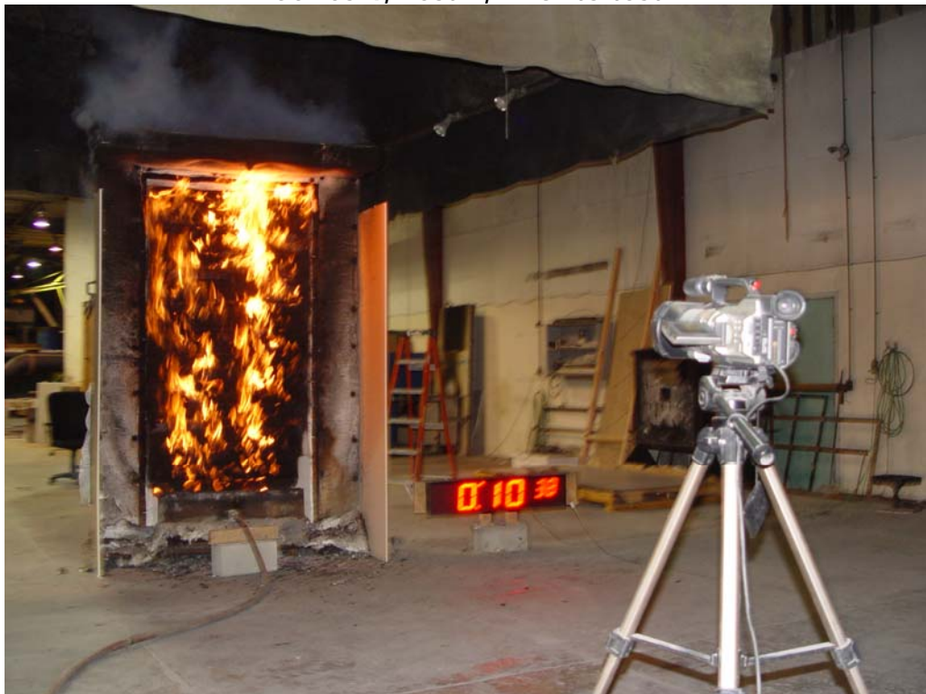
Series 4, Test 7, termination of burner at 10 minutes
