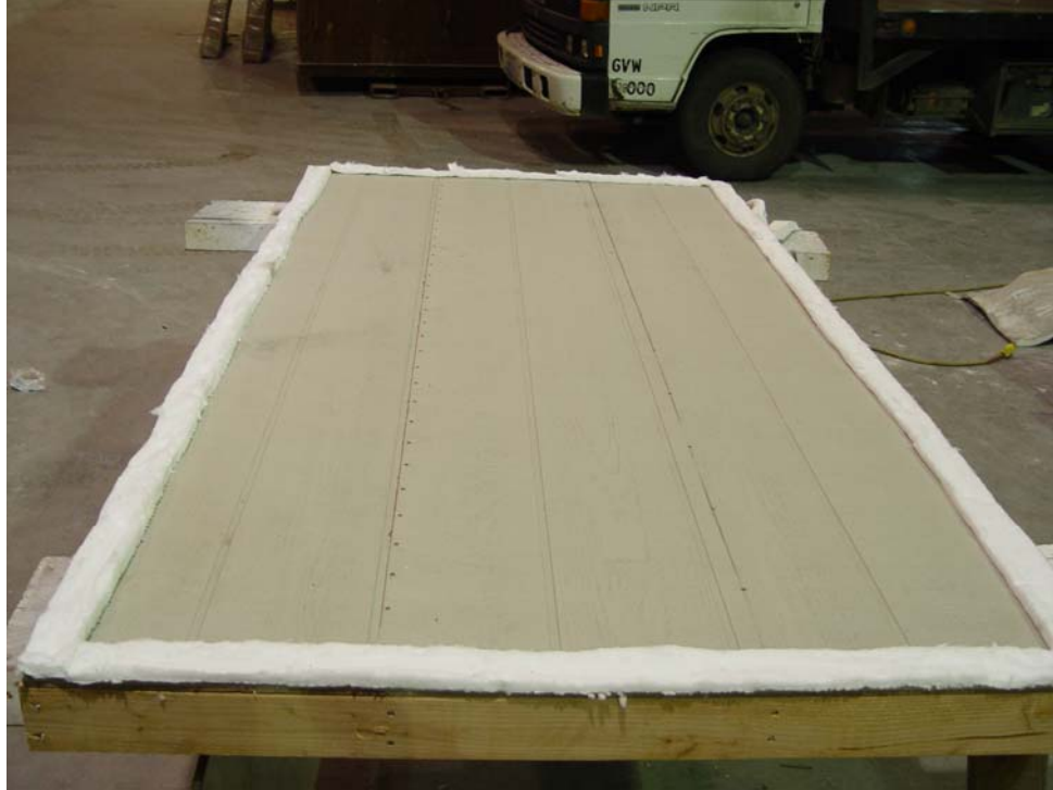
Test Series 2 , 7/16" LP Smartside® Foundation Series exterior panel siding – wet process fiber back-bone, with fire retardant seal (UL listed fire caulk, nominal ¼" bead) in the vertical joint, 3-in. nail spacing on the joint, 8" nail spacing in the perimeter and field (reference WFCi P/N 07028, Tests 7, 8 and 9)
