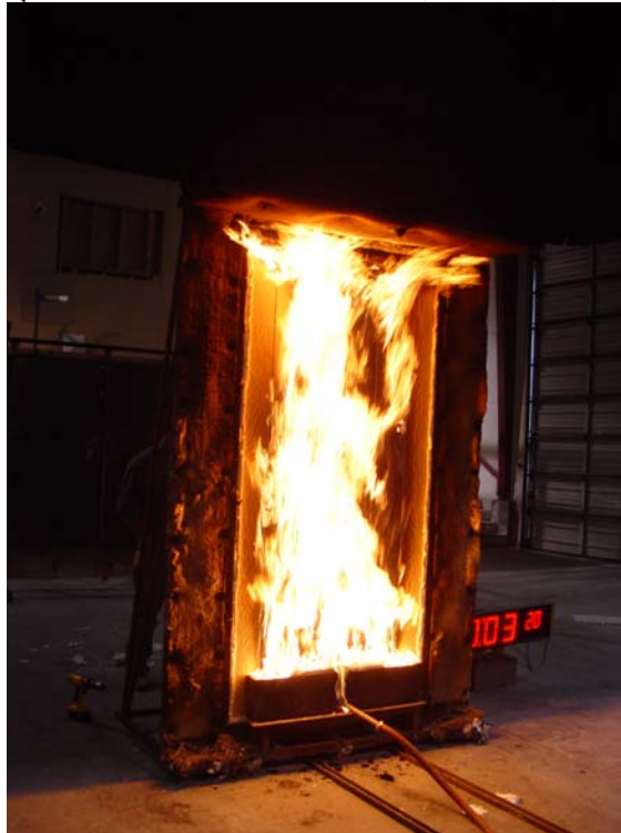
Test Series 1 , 7/16" LP Smartside® Precision Series exterior panel siding – oriented strand back-bone, with fire retardant seal (UL listed fire caulk, nominal 1/4" bead) in the vertical joint, 3-in. nail spacing on the joint, 8" nail spacing in the perimeter and field (reference WFCi P/N 06089, Tests 6, 8 and 9)
