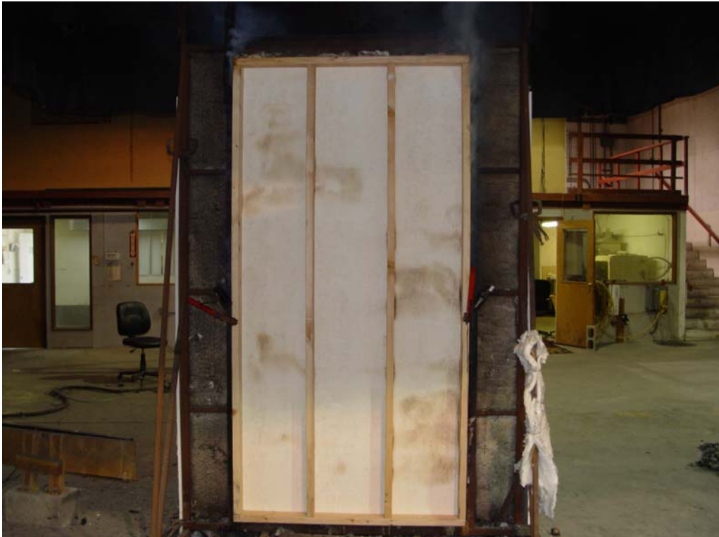
Series 4, Test 7, nonfire side at test termination (70 minutes)
