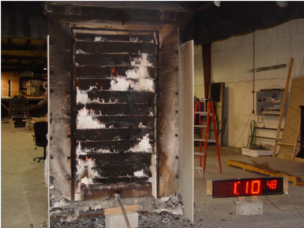
Series 4, Test 7, fire side at test termination
