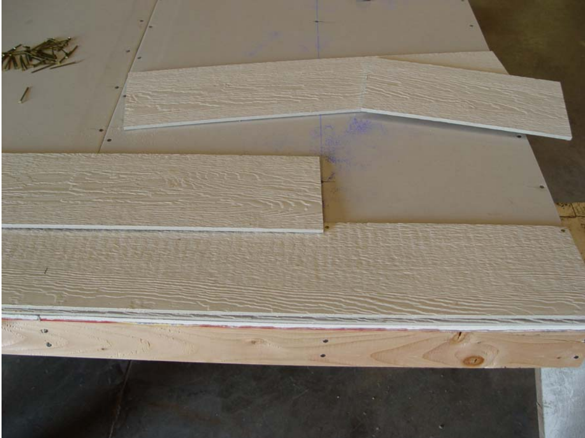
Test Series 3, 3/8" LP Smartside® Precision Series exterior lap siding – oriented strand back-bone, 8" wide, 1" overlap, 16" blind nailing, applied over 1/2" standard gypsum wall board substrate(reference WFCi P/N 07058, Tests 1,3 & 4)
