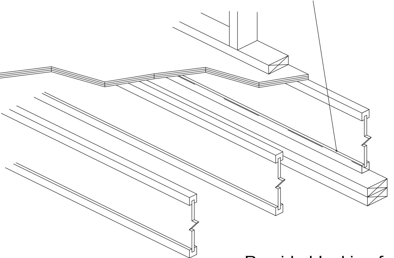
Provide blocking for lateral support as required. Use LP I-Joist, LP LVL, LP LSL, or LP Rim Board as blocking
