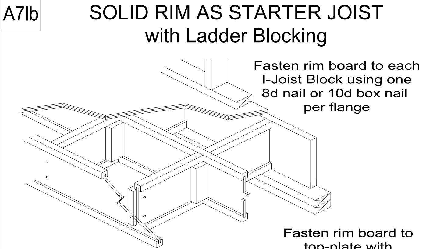
Fasten I-Joists to Connection Block with two (2) 8d box nails through the web and into the block. Fasten rim board to top-plate with 8d nail at 6" o.c.
