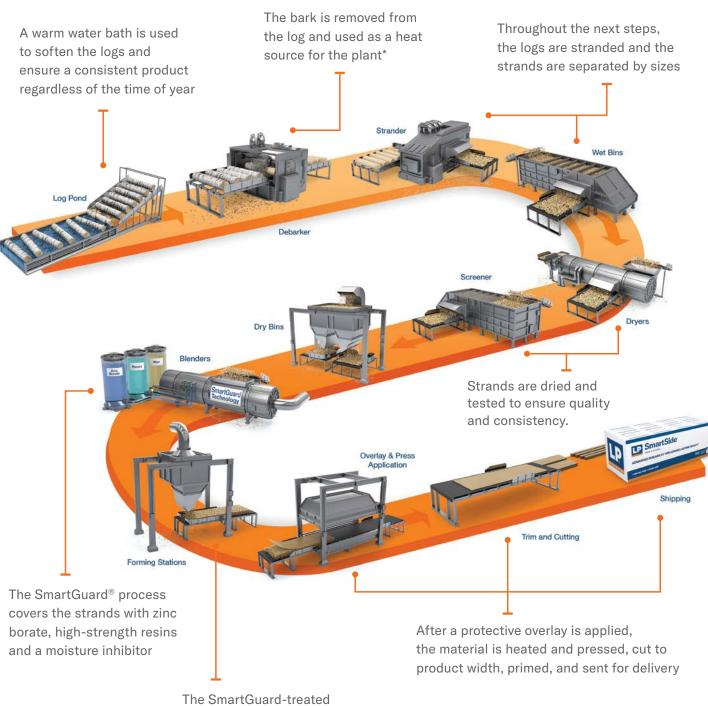
The SmartGuard-treated strands are then specifically oriented/layered for one of the most durable products available
