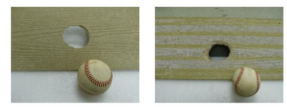
Figure 9. Posttest front (left) and rear (right) photos of FC panel impacted by a baseball in test LVG733
