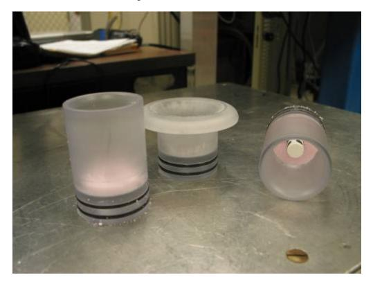
Figure 5. Typical polycarbonate sabots used for impact testing in the 2" bore gun. Sabot in center shows typical post-test geometry.
