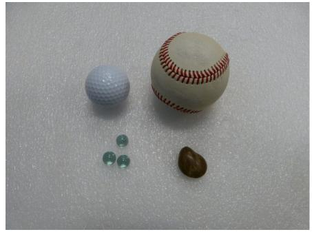
Figure 2. Projectiles used in impact tests
