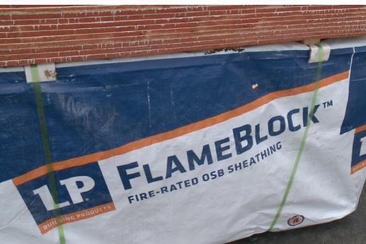
That’s because LP FlameBlock sheathing is designed to withstand exposure to moisture during normal construction delays, as evidenced by its Exposure-1 classification. The Grove at the Arboretum is a 112-unit development. Each condominium runs on
