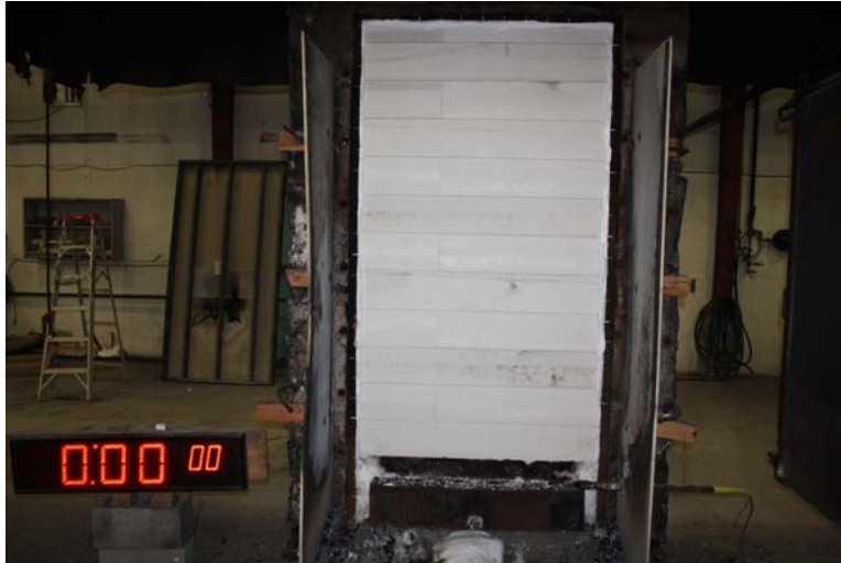
Test Series No. 1: Completed test assembly – Lap Siding
