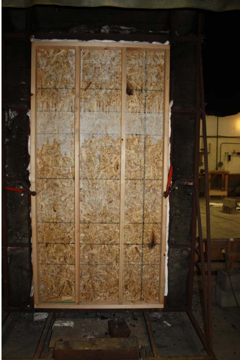
Unexposed side at test termination
