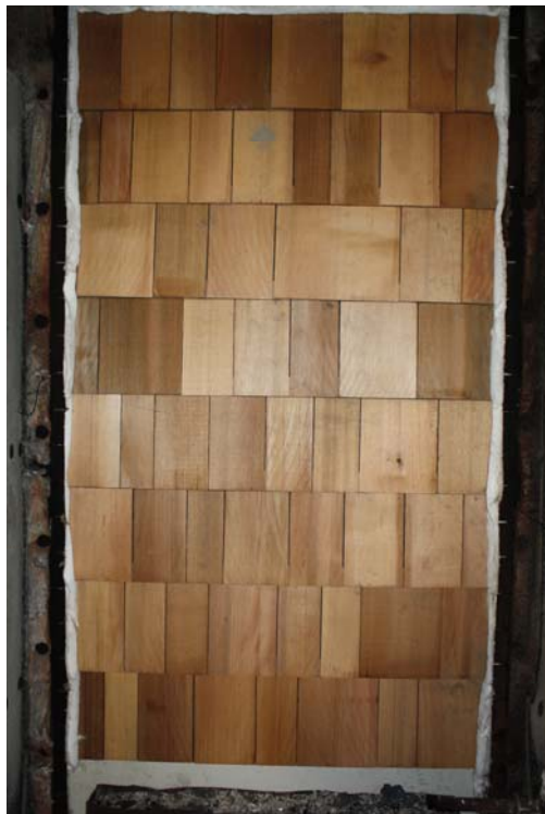
Test Series No. 2: Completed Wall Assembly
