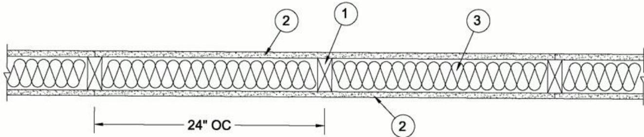
**1. Wood Studs** — Nom 2 by 6 in., spaced 24 in. OC with double 2 by 6 top and single 2 by 6 in. bottom plates. Studs effectively firestopped.
