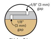
Shiplap Edge without Alignment Bead Figure 2b
