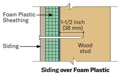
Siding over Foam Plastic Sheathing to Wood Studs
