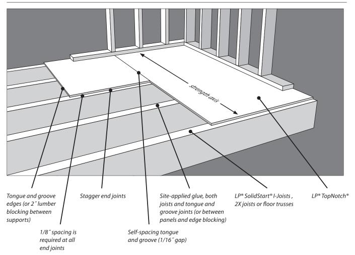
**Note:** Provide adequate ventilation and use ground cover vapor retarder in crawl space. Panels must be dry before applying finish flooring
