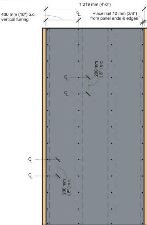
Min. 0.113 inch diameter **ring shank** hot-dip galvanized nail
