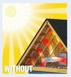
LP® TechShield® Radiant Barrier Sheathing blocks up to 97% of the radiant heat in the panel from entering into the attic.
