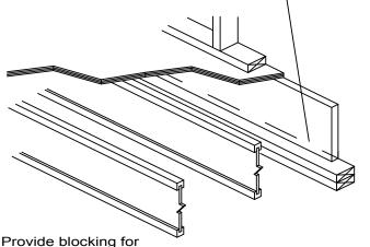
lateral support as required. Use LP I-Joist, LP LVL, LP LSL, or LP Rim Board as blocking
